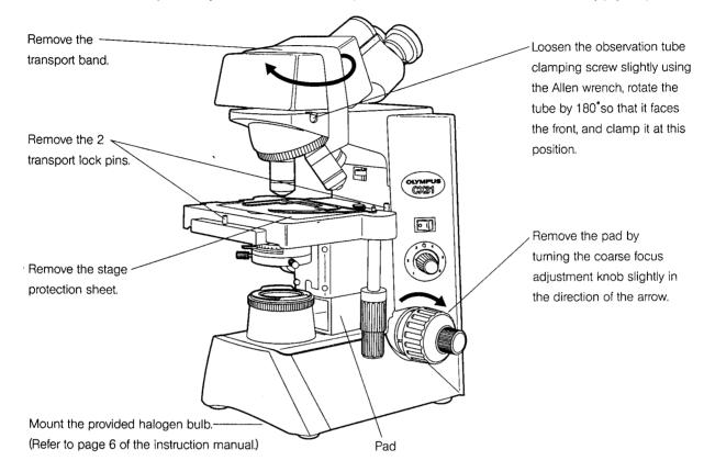
©The package includes the Instruction Manual, halogen bulb (6V, 30W), Allen wrench and immersion oil (when you purchase a 100X objective) as well as the CX31 microscope frame.
